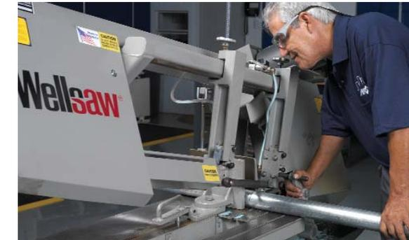
Frank Viscaino, Sr. cutting Schedule 40 solid bar stock for a shaft on the Variable Speed Wellsaw.
