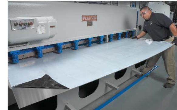
Rafael Sandoval shears a large sheet of stainless for recladding interior doors on the Heavy-Duty Mechanical Shear.
