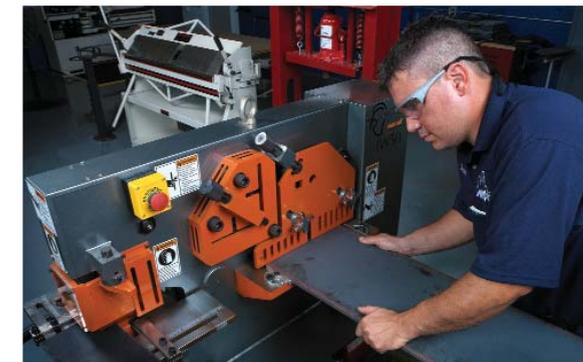
Frank Viscaino on the Hydraulic Ironworker shearing stainless steel. Box and Pan Brake shown in background.
